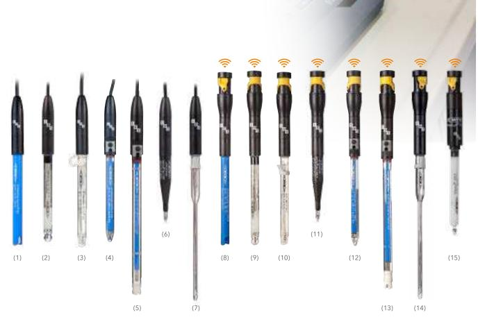
from left to right: the digital IDS sensors (1) SenTix® 940, (2) SenTix® 945, (3) SenTix® 950, (4) SenTix® 980; the IDS special electrodes (5) SenTix® HW-T 900, (6) SenTix® Sp-T 900, (7) SenTix® Micro 900; the wireless ready IDS plug head electrodes (8) SenTix® 940-P, (9) SenTix® 945-P, (10) SenTix® 950-P, (11) SenTix® Sp-T 900-P, (12) SenTix® 980-P, (13) SenTix® HW-T 900-P, (14) SenTix® Micro 900-P and (15) SensoLyt® 900-P
